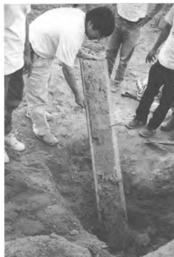
Photo 23. The soil peel is pulled away from the wall holding it with the plywood board.
