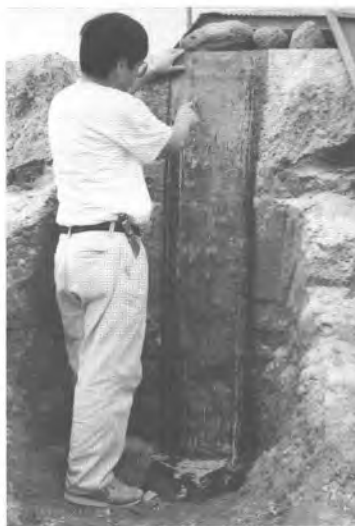
Photo 20. After hardening, the soil peel monolith to take is marked on the cloth.
