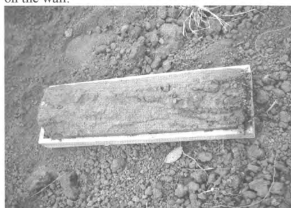
Photo 7. After cutting roots, the box is detached from the wall.
