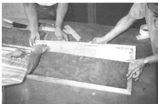
Photo 14. The peel is slipped into the mounting board.
