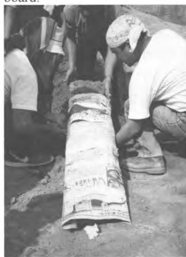
Photo 24. The soil peel is packed and transported to the laboratory.
