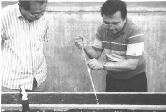
Photo 16. The diluted Bond CH18 emulsion is drop on the peel.
