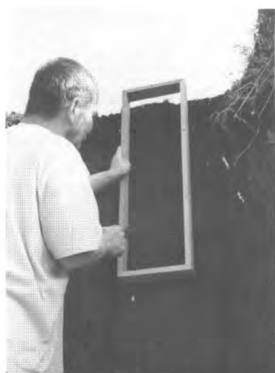
Photo 2. The internal dimensions of the monolith box are marked with a kitchen knife on the wall.
