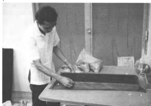
Photo 10. A piece of the cloth is put over the profile.
