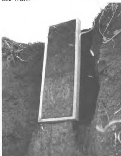
Photo 4. The box is pushed over the column.
