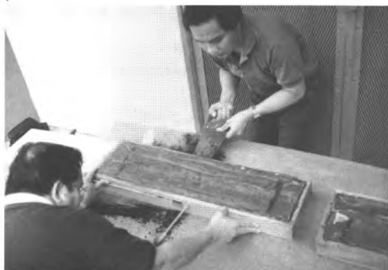
Photo 12. After hardening, the soil peel is cut off.
