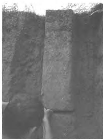
Photo 3. A soil column which has the exact internal dimensions of the box is cut on the wall.
