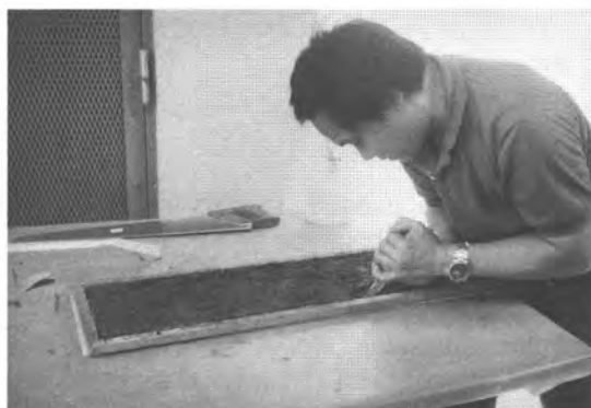
Photo 13. The bound frame is separated from the soil peel.
