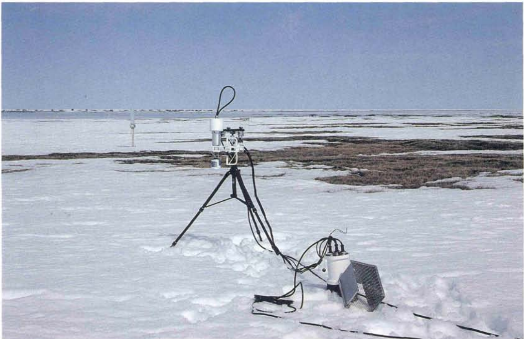
Photo. 8 Measurements of fluxes of \text{CO}_2 , latent and sensible heat by the eddy correlation measurement on snow covered tundra near DMCL/NOAA (June 8, 1993).
