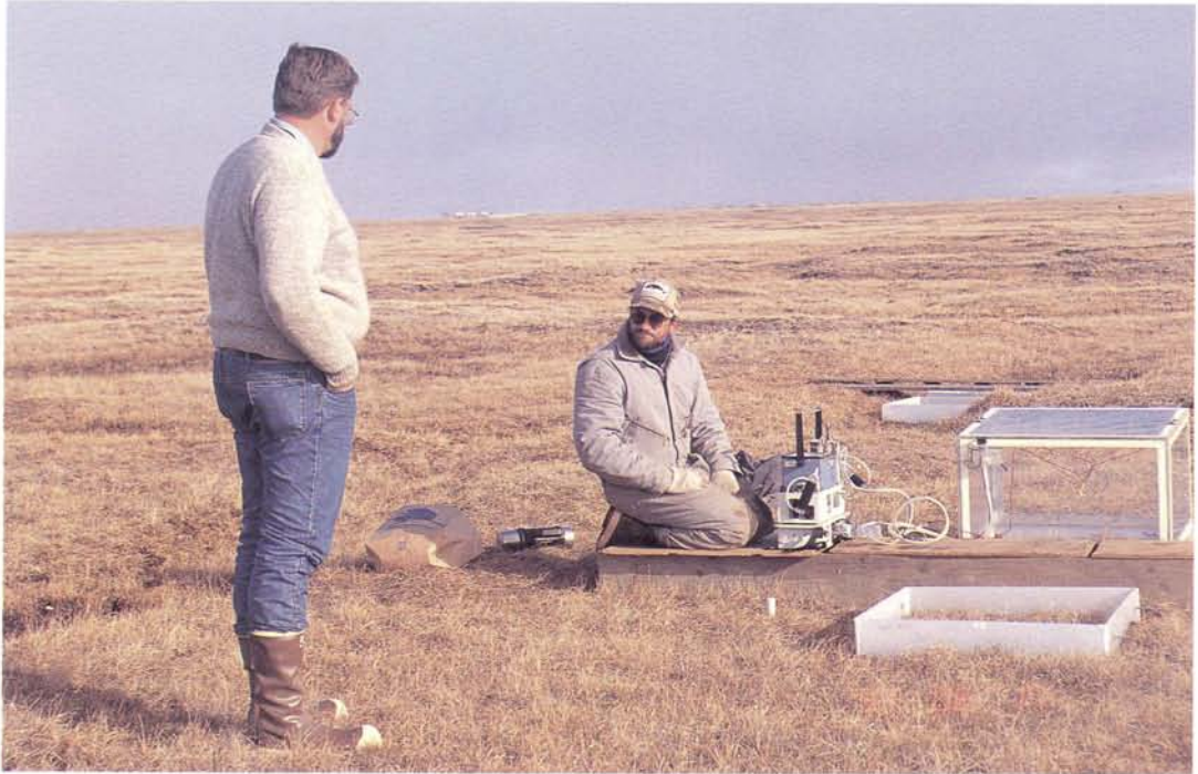
Photo. 12 CO 2 flux measurement at the IBP site using a chamber by the San Diego State University group.
