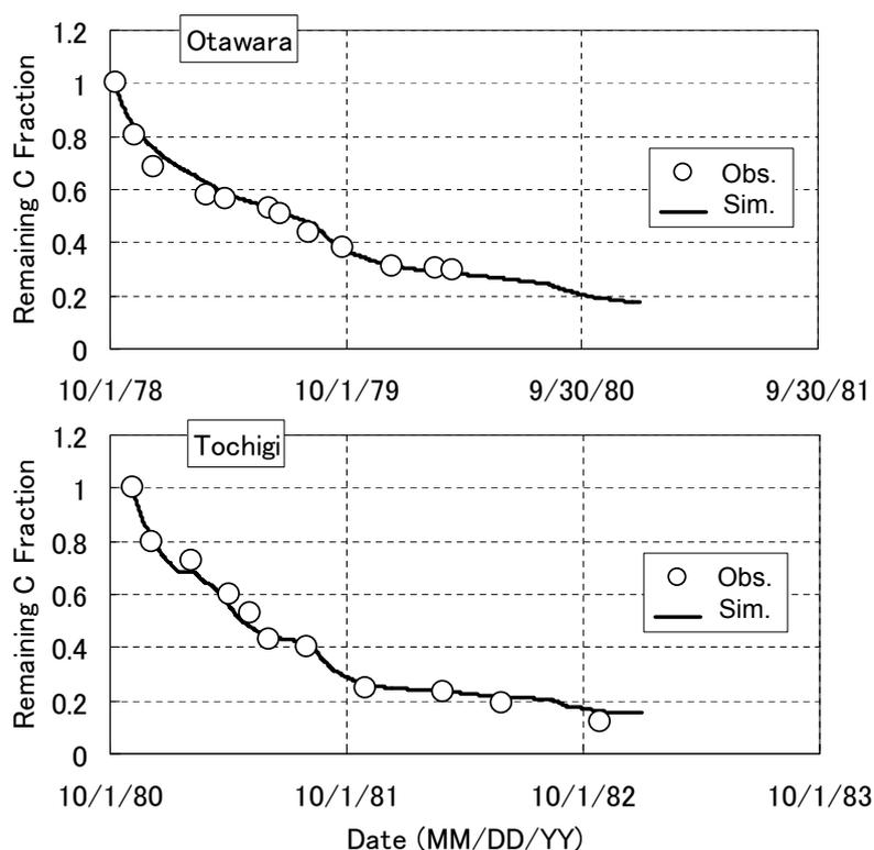
Fig. 5. Observed and simulated straw decomposition rates at two paddy fields in Tochigi prefecture, Japan. Observed data of straw decomposition were compiled from Mogi et al. (1980) and Yoshizawa and Nakayama (1983).
