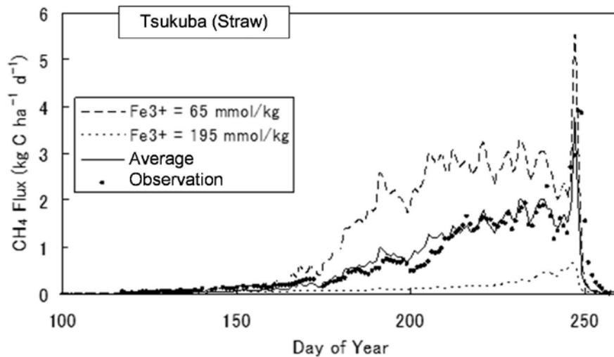
Fig. 11. Simulated daily  $\text{CH}_4$  fluxes from the Straw plot at the Tsukuba site, assuming a hypothetical heterogeneous soil system. The soil was assumed to consist of regions with different concentrations of reducible Fe (65, 130 and 195  $\text{mmol kg}^{-1}$ ), and the solid line represents the average of daily methane fluxes from those regions. Simulated methane flux assuming reducible Fe of 130  $\text{mmol kg}^{-1}$  is shown in Fig. 3.4a.
