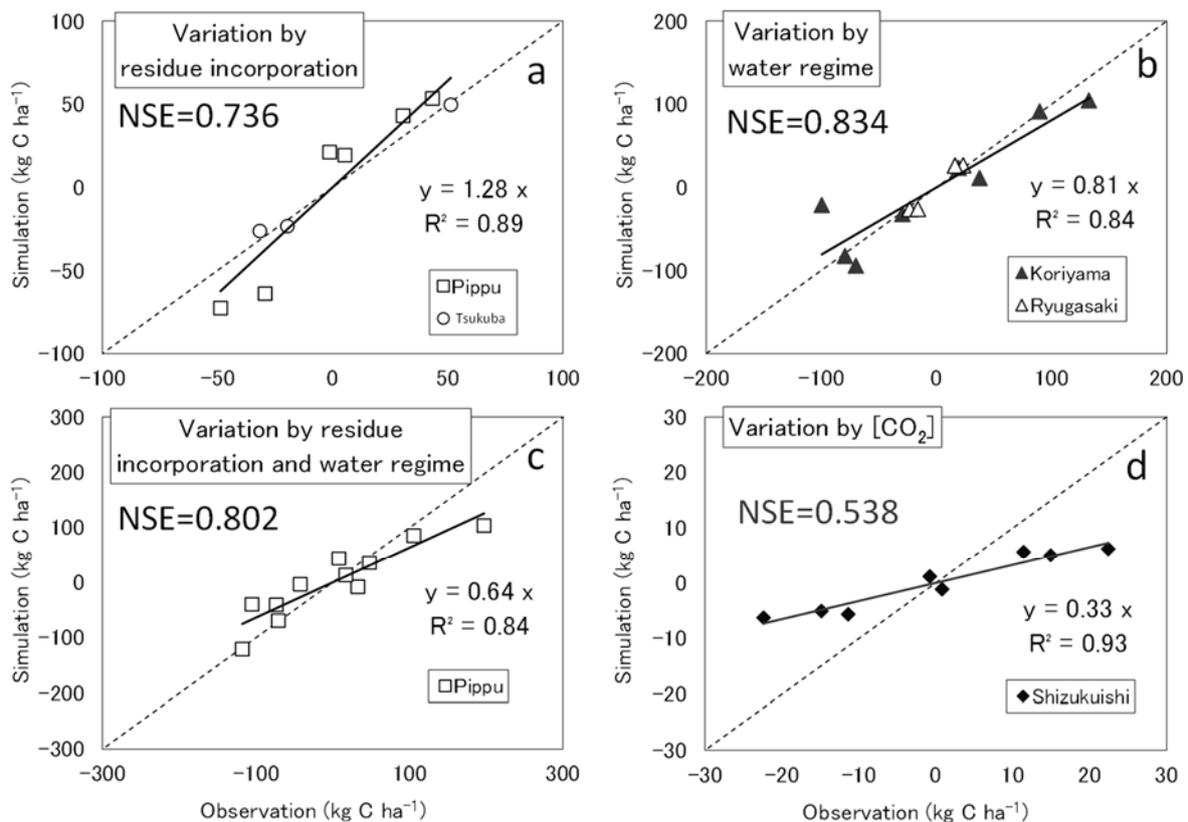
Fig. 8. Observed versus simulated variations in seasonal  $\text{CH}_4$  emissions due to different treatments of (a) rice residue incorporation, (b) water management, (c) combination of residue incorporation and water management, and (d) atmospheric  $\text{CO}_2$  concentration. Values of the x and y axes represent the difference from the mean of seasonal  $\text{CH}_4$  emissions across all treatments at each site in each year (refer to equation 3.2 in the text).
