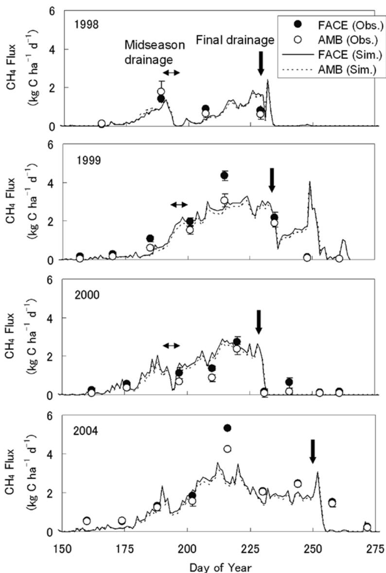
Fig. 22. Observed and simulated daily  $\text{CH}_4$  fluxes under elevated  $[\text{CO}_2]$  (FACE) and ambient  $[\text{CO}_2]$  (AMB) at the Shizukuishi site. Values of observed flux represent means  $\pm$  standard errors of the mean ( $n = 4$ ). Horizontal and vertical arrows represent the midseason drainage and the date of the final drainage, respectively. Observed data for years 1998-2000 were compiled from Inubushi et al. (2003).
