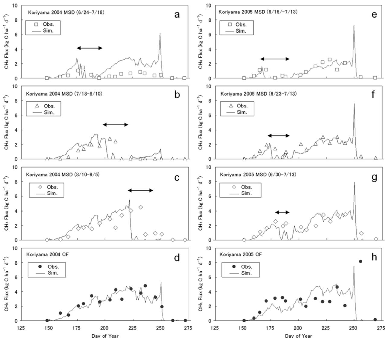
Fig. 12. Observed and simulated daily  $\text{CH}_4$  fluxes from the Koriyama site under different durations or timings of midseason drainage in 2004 (a-d) and 2005 (e-h). CF and MSD stand for continuous flooding and midseason drainage, respectively. The dates in parentheses represent the month/day of the start and end of midseason drainage, and horizontal bars ( $\longleftrightarrow$ ) indicate the periods of midseason drainage. Observed data were compiled from Saito et al. (2006).
