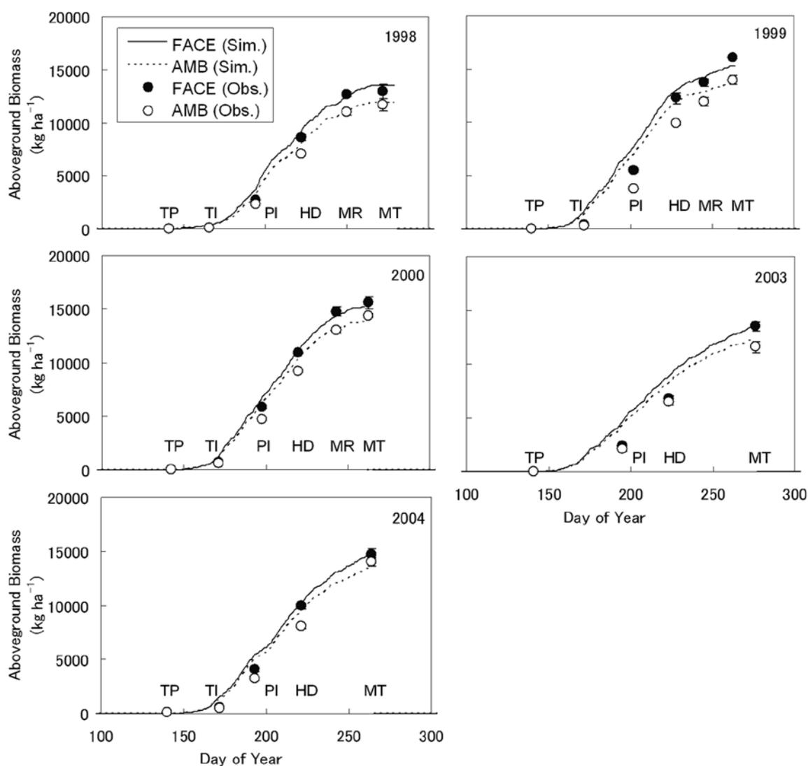
Fig. 19. Observed and simulated aboveground biomass under elevated  $[\text{CO}_2]$  (FACE) and ambient  $[\text{CO}_2]$  (AMB). Values represent means  $\pm$  standard errors of the mean ( $n = 4$ ). Rice plant developmental stages on each sampling date are as follows: TP, transplanting; TI, tillering; PI, panicle initiation; HD, heading; MR, mid-ripening; MT, maturity. Observed data were compiled from Kim et al. (2001, 2003).
