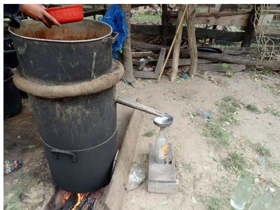
Photo 15. Traditional method of making distilled liquor from rice in the Donghongkham village
