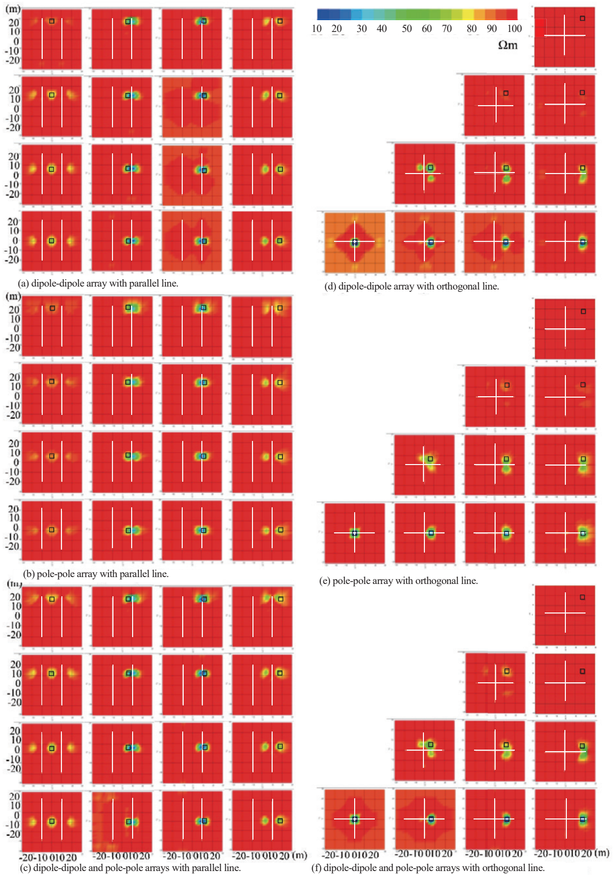
Fig.30 A resistivity slice at depth of 4 m reconstructed from 3D inversion of synthetic data obtained along two parallel lines (a, b and c) and two orthogonal lines (d, e and f). The square black box shows the location of the conductive body in the half-space.
