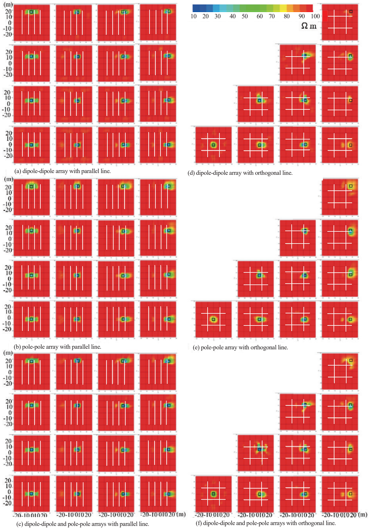
Fig.31 A resistivity slice at depth of 4 m reconstructed from 3D inversion of synthetic data obtained along four parallel lines (a, b and c) and four orthogonal lines (d, e and f). The square black box shows the location of the conductive body in the half-space.
