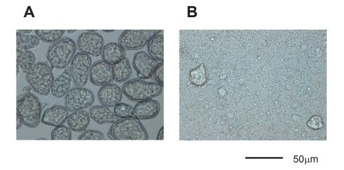
Fig. 1 Micrographs of Ann-paste preparation (left) and microground Ann particles (Right)
