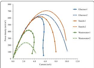
**Fig. 1** Power density of the MFCs equipped with FO-SSA using different substrates as fuel. Two reactors were operated for each substrate
