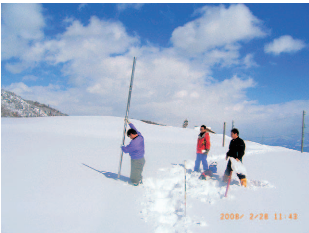
Fig. 37 A snow sampler being used during the snow survey.
