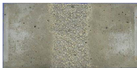
Fig. 42 試験終了後の試験体 (M40) Surface state of the specimen after erosion test (M40)
