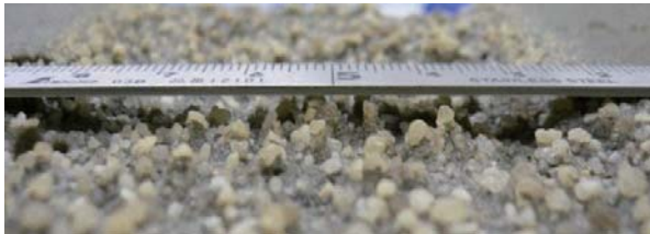
Fig. 47 M50 の摩耗状況 (28 日後) Eroded surface state of specimen M50 after test (28 days)
