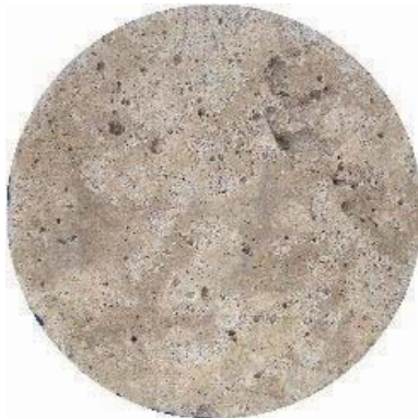
Fig. 87 E地区背面の状況 Back surface state of collected core in the E district
