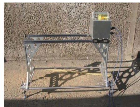
Fig. 9 摩耗形状計測装置 Measuring device for eroded surface profile
