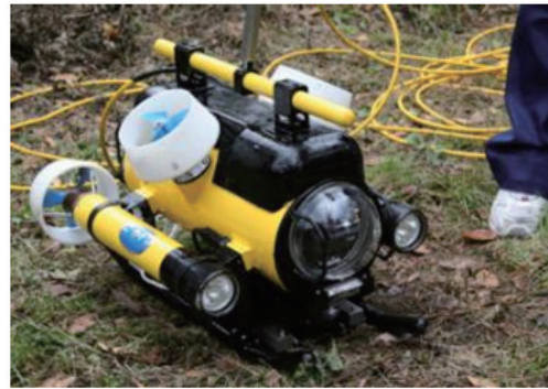
Fig.3-21 水中ロボットカメラ Remotely operated vehicle
