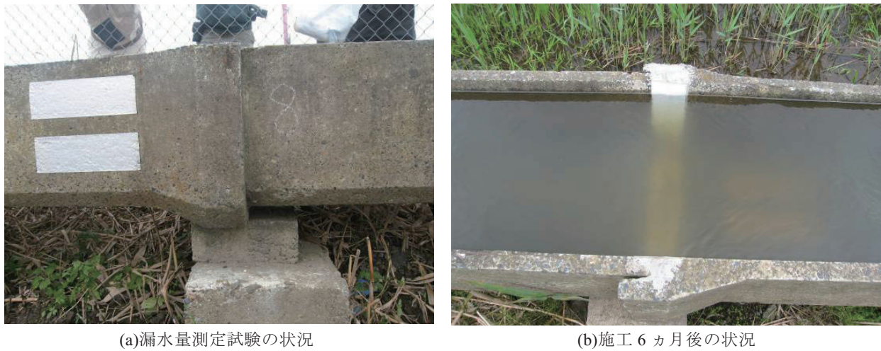
Fig.5-23 現地水路での止水性の確認状況 Water leak amount test in irrigation canal
