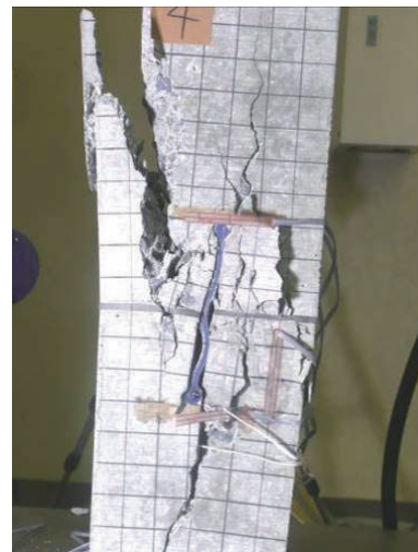
Fig.2-69 供試体4の試験後の破壊状況 Destruction situation of the test specimen4 after the loading test
