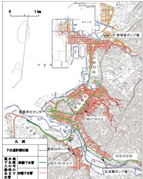
Fig.14 塩水地下水浸入の可能性のある下水管の分布状況 Distribution of sewer pipes having possibility of saline groundwater infiltration
