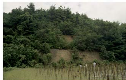
Fig.28 肥料袋工追肥試験区設定法面の変化 Change of the slope of topdressing by fertilizer bags
