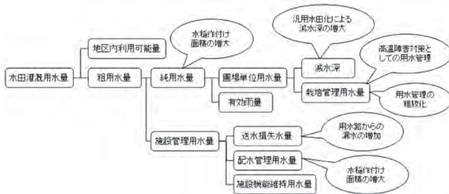
Fig.5 水田灌溉用水量の構成と水田農業の営農変化に伴う影響 Components of paddy field irrigation water and impacts of rice production changes
