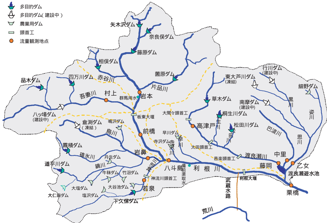
Fig.3 利根川上流域における水資源施設 (多目的ダムまたは農業用ダム堤高15m以上, 主要取水施設等) Water resource facilities in the Upper Tone River Basin (Multi-purpose dams and/or agricultural dams with dam height of 15m or more, and main intake facilities)
