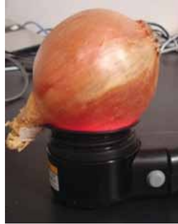
Fig. 3 The measurement of the NIR spectrum of an onion using the K-BA100R spectrophotometer. The onion is being illuminated with the NIR beam.
