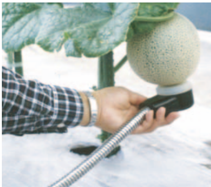
Photo.1 Non-destructive determination of Brix in a growing melon using Near Infrared spectroscopy (image)
