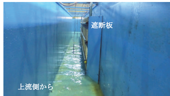
Fig. 11 EM 上流端の遮断板 Outline of shutdown plate at the upstream end of expanded metal
