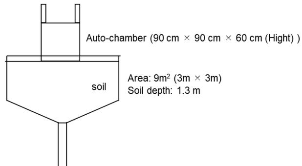
c. Schematic diagram of automated flux monitoring system
