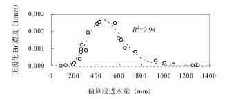
Fig.13 浸透水中の臭化物イオン濃度の推移 Br- concentration in leachate
