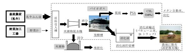
Fig.15 温室効果ガス排出量を算定する範囲 System boundary for calcurating greenhouse gas emissions
